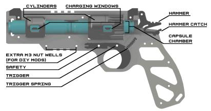
cylinder may be needed if the fit is too tight. Cylinders should stay in place with a light friction fit, with the charging ports aligned with the charging windows. A loose fit is okay - the ports may just need occasional realigning.
