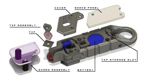
3. Remove the snake panel to access the battery. You may need a flathead screwdriver to pry the battery out.
